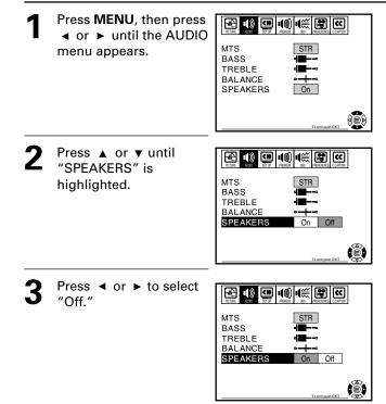
**To turn on the built-in speakers** Select "On" in step 3.
